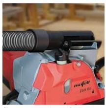
Since a large volume of chips can be produced at cutting depths of up to 400 mm (15 3/4 in.), the ZSX-TWIN Ec can also be used in conjunction with an extraction system.
