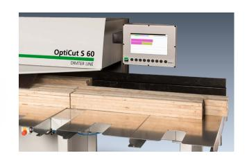
The perfect solution for 1-man-operation. The finished parts are lying next to each other in the cut sequence at the outfeed of the saw. This means very short distances for the operator to carry out destacking (e. g. while the machine is treating the next workpiece).
