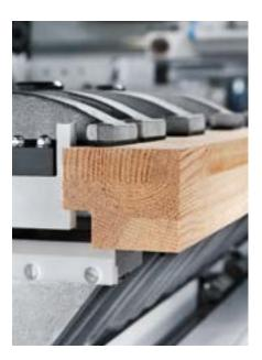
**PowerGrip clamping table and U-axis** The interaction of the patented PowerGrip clamping table, U-axis, workpiece measurement (optional) and alignment of the parts ensures superior process reliability.
