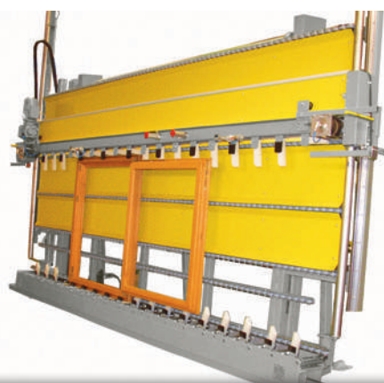
RU-SE-HA // Lifting station with clamping unit from above
