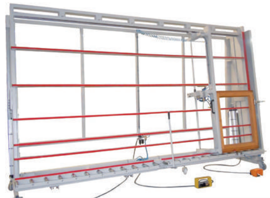
RU-VGP-WR // Glazing and control press with 90° turning unit
