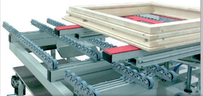
RU-ST-DH // Sliding table with turn lift devices
