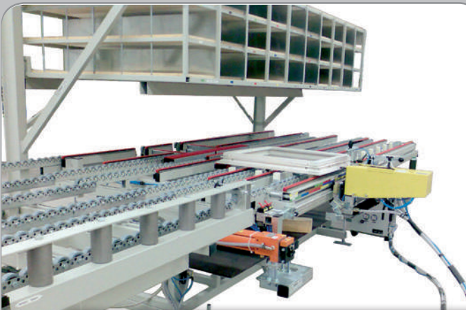
RU-BM // Sash hardware assembly table with roller ledges that can be raised and lowered
