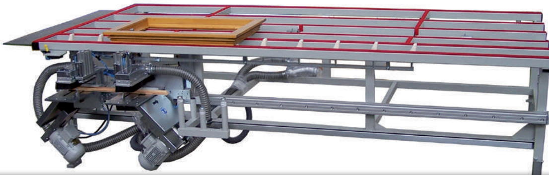
RU-GL-45° // Double glazing bead saw with length gauge on the sliding working table
