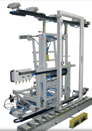
RU-MKS // Tilt table with clamping device and 83° to 90° tilt position
