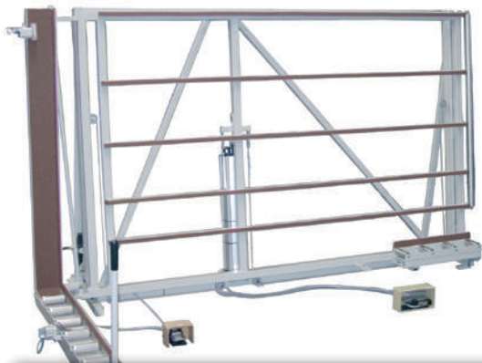
RU-SW 90° // Lifting station with 90° turning unit
