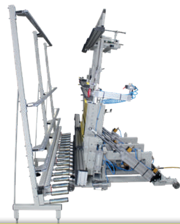
RU-MKSE-P4R // Roller shutter box assembly table, with pneumatically height-adjustable platform and transfer roller conveyor. Bearing capacity 400 kg
