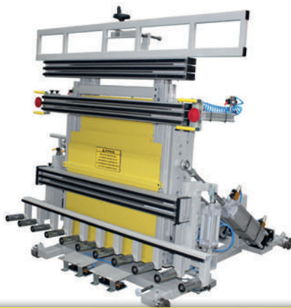
RU-MKSE-P4R // Roller shutter box assembly table, with pneumatically height-adjustable platform and transfer roller conveyor. Bearing capacity 400 kg
