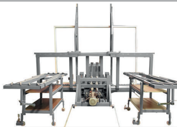
RU-MSA-K // Hydraulic lift tilt device for façade elements up to 1000 kg
