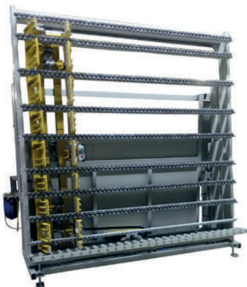
RU-FSPAI // Sash press with inner and outer clamping
