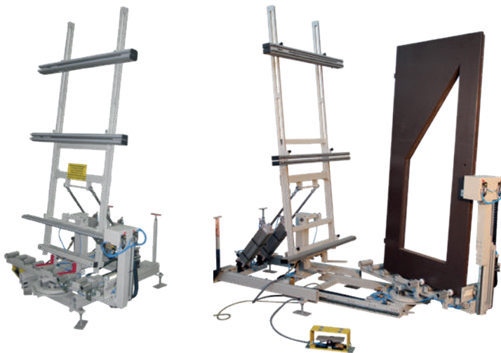
RU-TMK // Tilt table with 360° rotary mechanism
