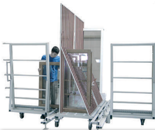
RU-FPA // Sash buffer with a movable in-feed and outfeed roller conveyor
