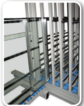
RU-P-ES // Glass buffer with an movable outfeed roller conveyor
