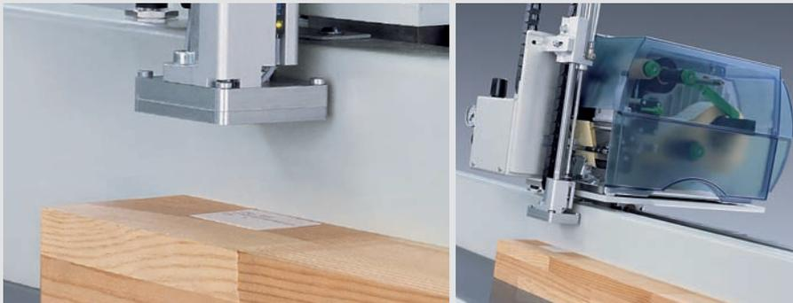
With the **label printer** labels can be generated and applied fully automatically, with the printer being completely integrated into the control of the OptiCut S 90. Due to the bar code, the identification of the piece becomes even machine-readable and further machines in the production process can even adapt themselves correspondingly to the workpiece. Individual designs of the labels are no problem in this situation.
