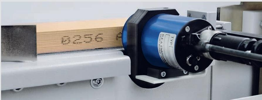
For the clear identification of the pieces after the cutting, inkjet or label printers are used.
