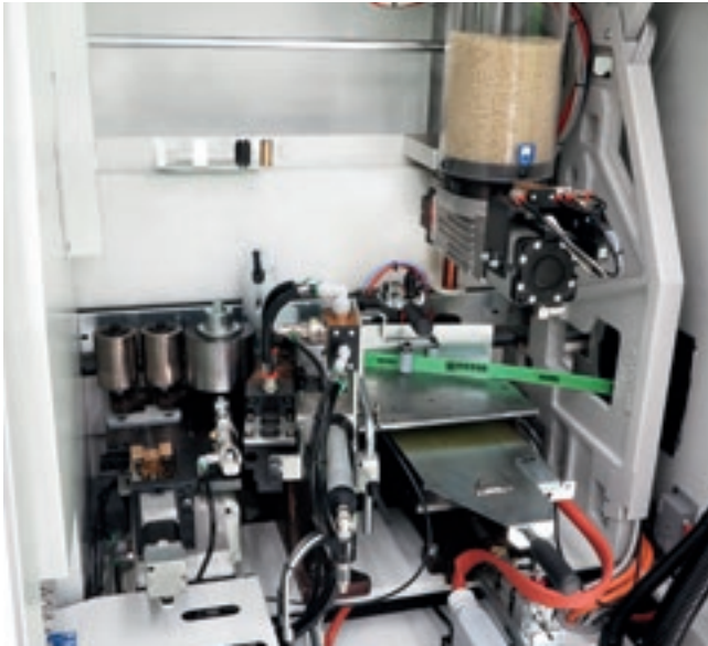
Gluing unit for the automatic application of edging in rolls or strips, from 0.4 to 12mm.
