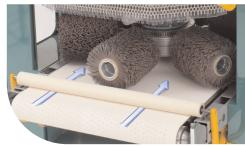
The strong, compact gear head is equipped with a total of six spindles, mounted in pairs, rotating alternately clockwise and counterclockwise.
