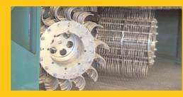
Removal of slags on the surface after plasma cutting: Heavy duty tool that knocks off the large burrs on the edges.
