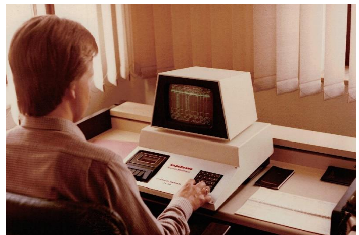
PET 2000 – the world's first computer control system for lumber drying
