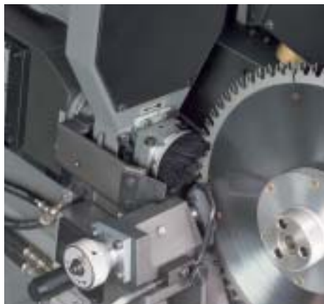
Hollow face grinding device as optional extra
