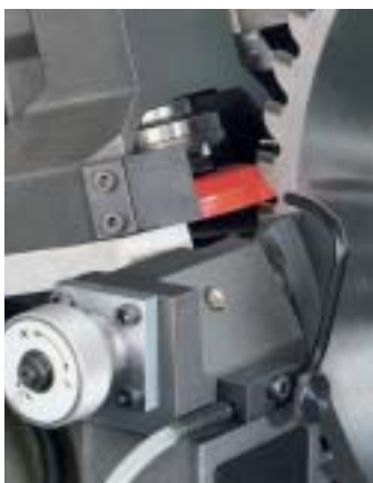
For tooth shapes with negative hook angles of up to 20°
