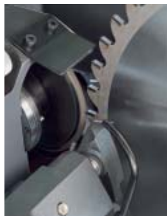
Option: grinding of a chip breaker groove of TCT or HSS saw blades
