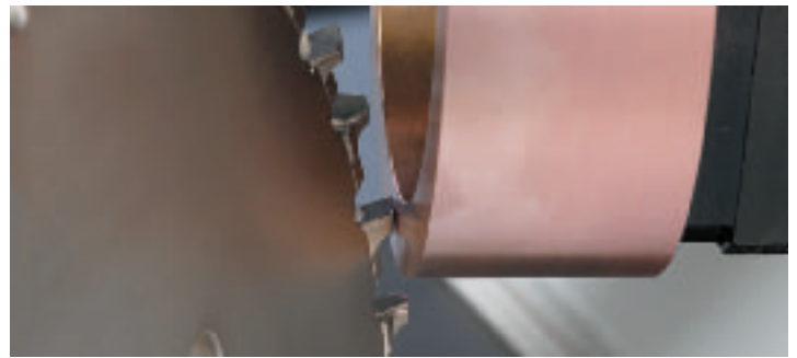
Hoggers with freely programmable tooth profiles
