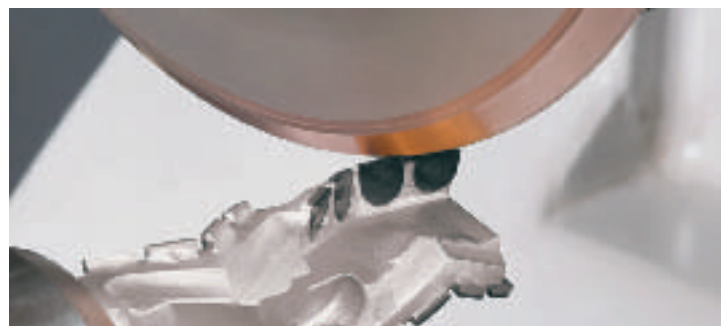
Milling cutter with tothing on left and right-hand side
