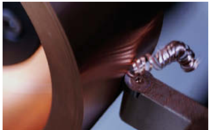
Dressing the eroding disc in the machine
