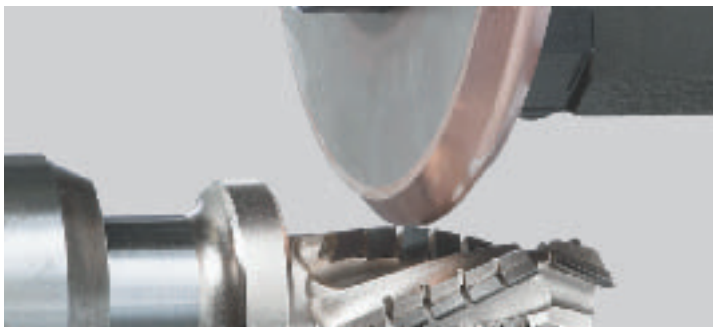
End milling cutter with several cutting edges and small clearances (speedy milling cutter)
