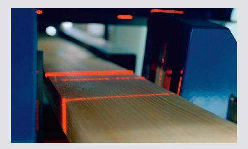
Scanner systems detect fully automatically and at lightning speed relevant workpiece characteristics such as branches, cracks and structural patterns, and supply up to 4 OptiCut high-speed saws with cutting data via intelligent mechanisms while maintaining full production speed.
