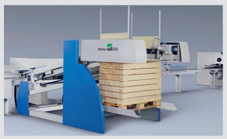
The **OptiCut Stacker** is the ideal solution for the production of preferred lengths. These are stacked fully automatically to a stacking height of 1200 mm and at a rate of up to 80 parts/min. Different stacking patterns can be selected in the saw control system.
