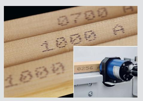
Easy handling of the sawn timber, warehouse identification, order-based assignment, product-based logistics – in all these cases, the identification of the cut lengths has an important role to play. Thus, a clearer overview, lower costs or in general the use of cost-optimised production processes are made possible. Number or code labelling is performed directly on the workpiece, from the side or above.
